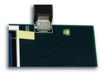
6. Using a metal object, short the *Firmware-Erase* pads to enable the USB Bootloader, then simultaneously reset the board using the reset switch on the bottom of the board.
