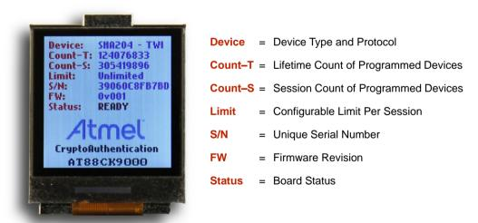
6. Congratulations, the AT88CK9000 board is up and running. You may now load the devices into the sockets and press the Program button when ready to program the parts.
