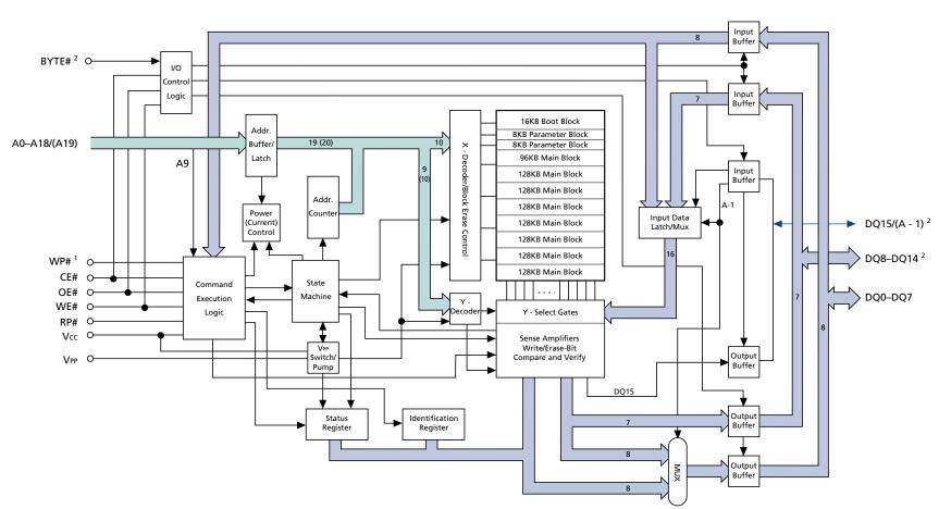
Figure 2: Functional Block Diagran
