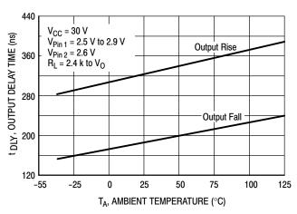
Figure 7. Uncommitted Comparator Delay versus Temperature
