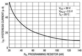
Figure 5. Power Warning Hysteresis Current versus Programming Resistor
