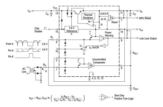
Figure 12. Line Loss Detector Application
