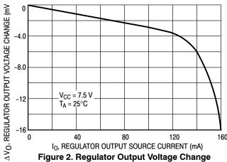
Figure 2. Regulator Output Voltage Change versus Source Current
