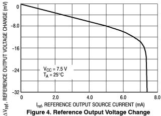
Figure 4. Reference Output Voltage Change versus Source Current
