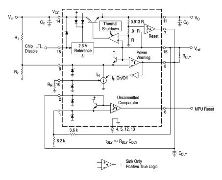
Figure 13. Time Delayed Microprocessor Reset
