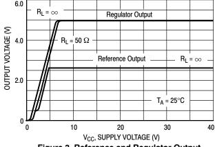
Figure 3. Reference and Regulator Output versus Supply Voltage
