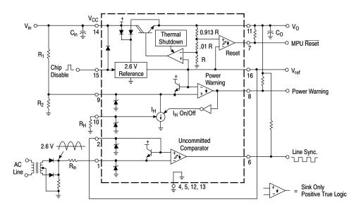
Figure 11. Typical Microprocessor Application
