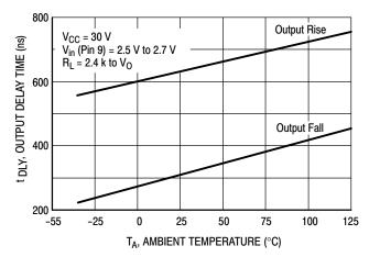
Figure 6. Power Warning Comparator Delay versus Temperature
