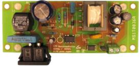
short-circuit protection, skip-cycle, a maximum peak current set point, ramp compensation, and a Dynamic Self-Supply (eliminating the need for an auxiliary winding).
