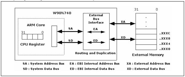
Fig. 7.2.4 Address/Data bus connection with external memory
