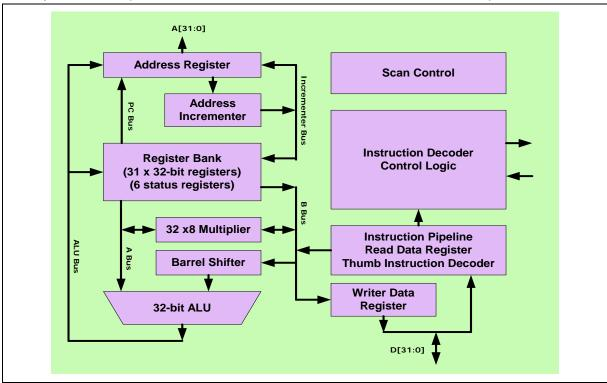
Fig 7.1 ARM7TDMI CPU Core Block Diagram
