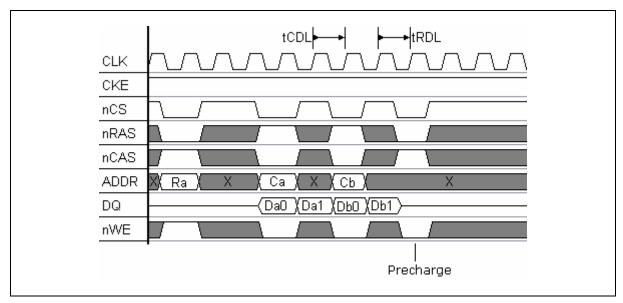
Fig 7.3.5 Access timing 2 of SDRAM
