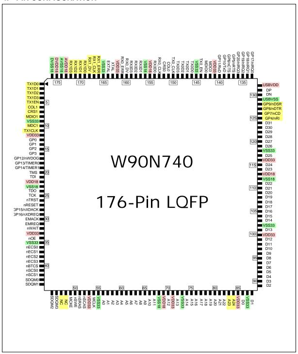
Fig 4.1 176-Pin LQFP Pin Diagram
