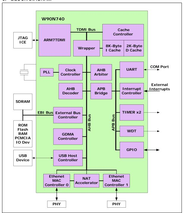
Fig 3.1 W90N740 Functional Block Diagram
