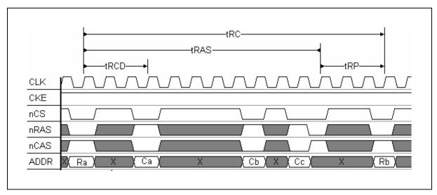
Fig 7.3.4 Access timing 1 of SDRAM
