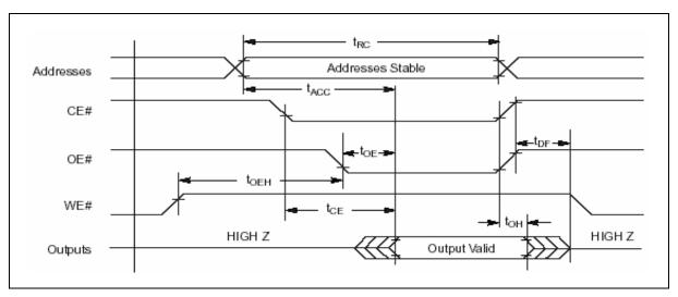
Fig7.3.2 ROM/FLASH Read Operation Timing
