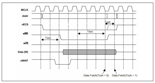
Fig 7.3.6 External I/O write operation timing
