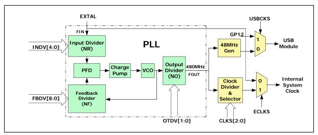
Fig 7.2.6 System PLL block diagram
