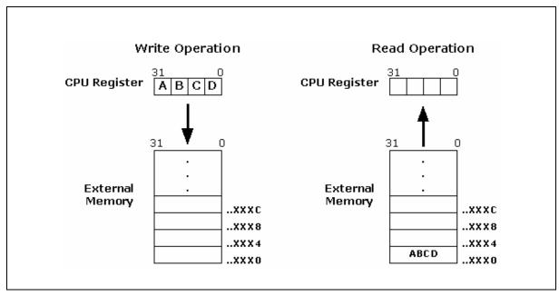
Fig. 7.2.5 CPU register Read/Write with external memory
