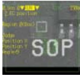
Positioning of PCB's Fiducial Marks
