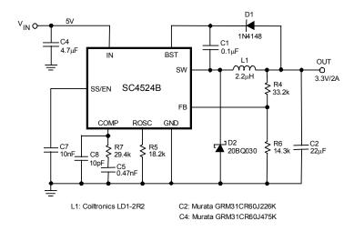
Figure 10. 1MHz 5V to 3.3V/2A Step-down Converter
