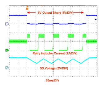
Figure 12(d). Output Short Circuit (Hiccup)
