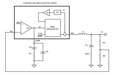
Figure 7. Block diagram of control loops
