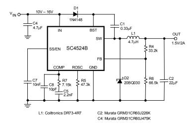
Figure 11. 500kHz 10V-16V to 1.5V/2A Step-down Converter
