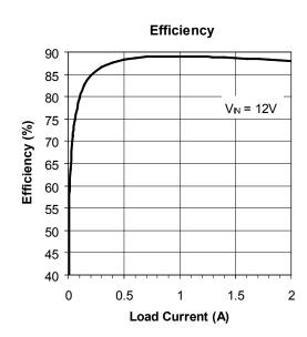
Figure 1. 1MHz 10V-16V to 5V/2A Step-down Converter
