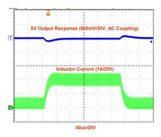
Figure 12(c). Load Transient Response  $(I_0 = 0.3A \text{ to } 2A)$
