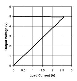
Figure 12(a). Load Characteristic
