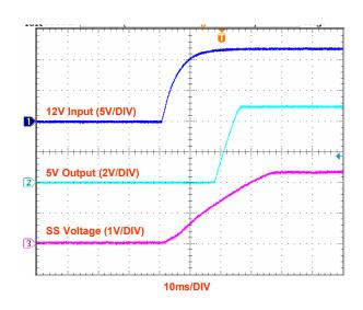
Figure 12(b).  $V_{IN}$  Start up Transient ( $I_{O}$ =2A)
