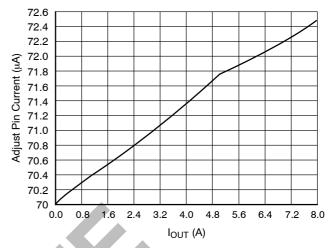
Figure 6. Adjust Pin vs. IOUT
