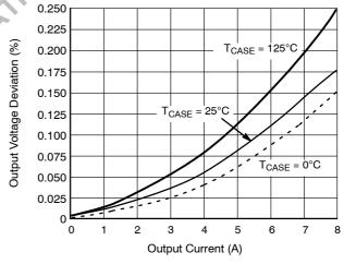
Figure 4. Load Regulation vs. Output Current
