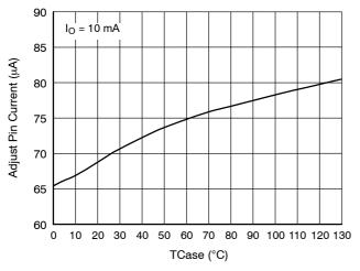
Figure 5. Adjust Pin Current vs. Temperature
