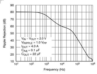
Figure 10. Ripple Rejection vs. Frequency
