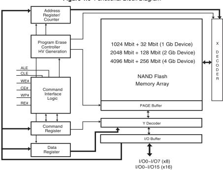
Figure 1.6 Functional Block Diagram
