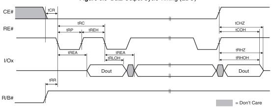
Figure 6.5 Data Output Cycle Timing (EDO)
