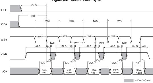
Figure 6.2 Address Latch Cycle
