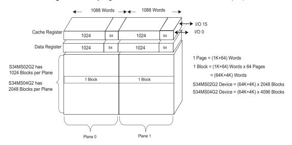
Figure 1.10 Array Organization — S34MS02G2 and S34MS04G2 (x16)
