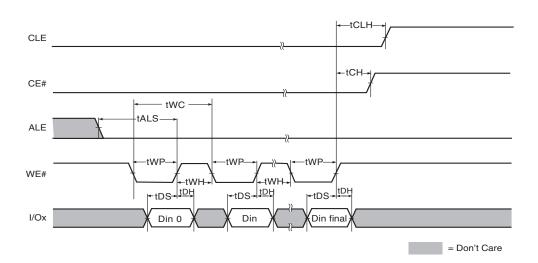
Figure 6.3 Input Data Latch Cycle
