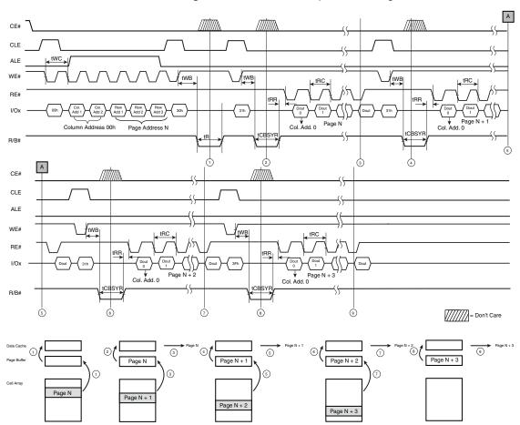
Figure 6.25 Read Cache Operation Timing
