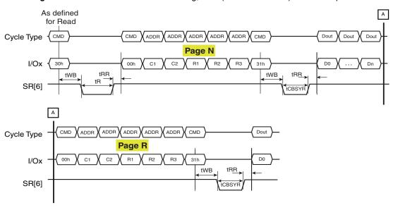
Figure 6.28 Read Cache Timing, End Of Cache Operation
