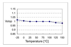
Figure 7. Stop Threshold Voltage
