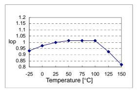
Figure 3. Operating Supply Current
