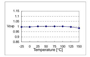
Figure 12. Over Voltage Protection
