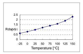
Figure 14. Static Drain-Source on Resistance
