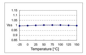
Figure 13. Soft Start Voltage
