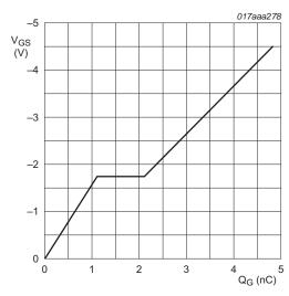
$I_D = -3 A$ ;  $V_{DS} = -10 V$ ;  $T_{amb} = 25 °C$
