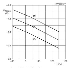
$I_D$  = -0.25 mA;  $V_{DS}$  =  $V_{GS}$
