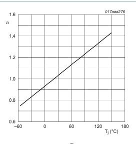
$$a = \frac{R_{DSon}}{R_{DSon(25^{\circ}C)}}$$
