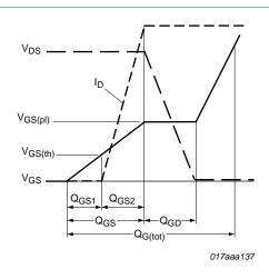
Fig 15. Gate charge waveform definitions
