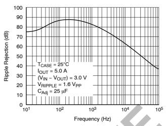
Figure 9. Ripple Rejection vs. Frequency (Adjustable Versions)
