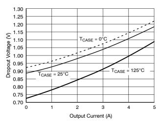
Figure 3. Dropout Voltage vs. Output Current
