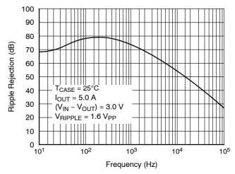
Figure 8. Ripple Rejection vs. Frequency (Fixed Versions)
