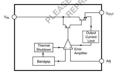
Figure 1. Block Diagram - CS5205-1
