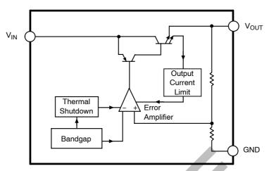
Figure 2. Block Diagram - CS5205-3, -5
