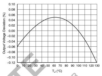
Figure 4. Reference Voltage vs. Temperature
