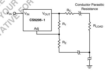
Figure 14. Grounding Scheme for Adjustable Output Regulator to Minimize Parasitics
