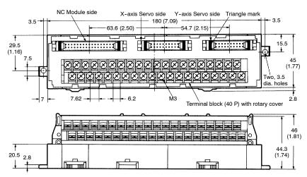
Note: The terminal block has a terminal pitch of 7.62 mm.
