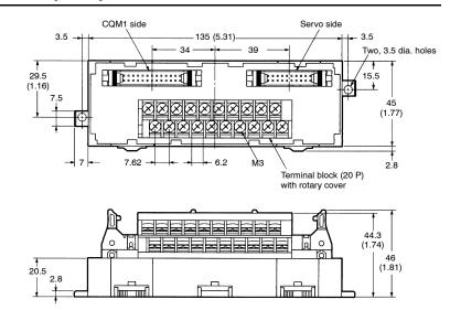
Note: The terminal block has a terminal pitch of 7.62 mm.
