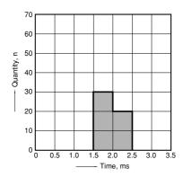
5. Distribution of release time Sample: JJM2W-12V, 50pcs. \* Without diode
