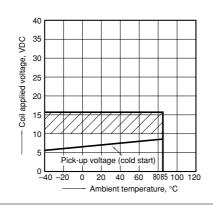
3. Distribution of pick-up and drop-out voltage Sample: JJM2W-12V, 50pcs.
