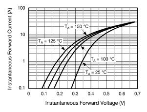
Fig. 3 - Typical Instantaneous Forward Characteristics
