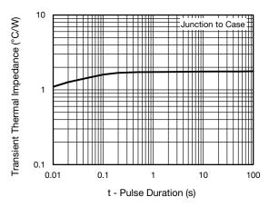
Fig. 6 - Typical Transient Thermal Impedance
