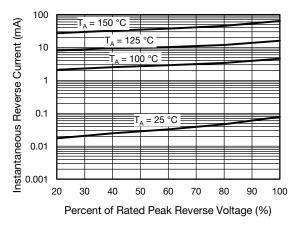
Fig. 4 - Typical Reverse Characteristics
