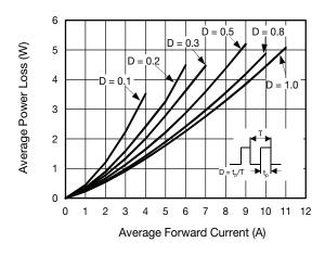
Fig. 2 - Forward Power Loss Characteristics
