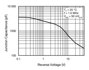
Fig. 5 - Typical Junction Capacitance
