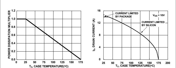
Figure 1. Normalized Power Dissipation vs Case Temperature
