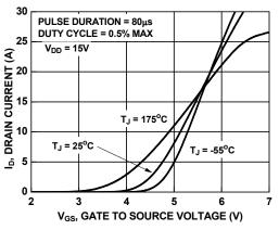
Figure 7. Transfer Characteristics
