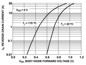
Figure 8. Forward Diode Characteristics
