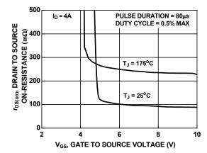
Figure 11. Rdson vs Gate Voltage
