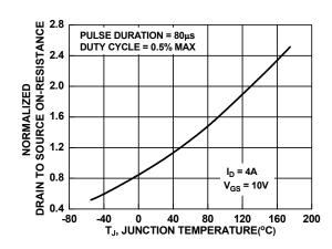
Figure 12. Normalized Rdson vs Junction Temperature
