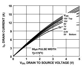
Figure 10. Saturation Characteristics
