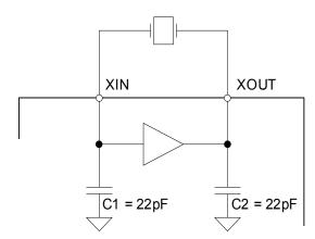
Figure 1. Oscillator Connections
