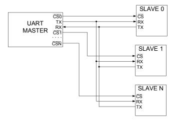
Figure 2. Multi-device UART Connections
