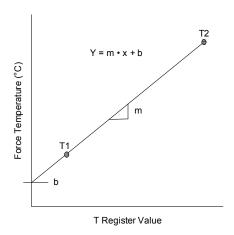
Figure 26. T Register vs. Force Temp
