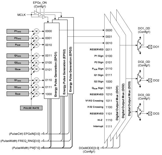
Figure 16. Energy Pulse Generation and Digital Output Control
