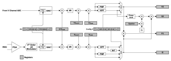
Figure 10. Signal Flow for V2, I2, P2, and Q2 Measurements
