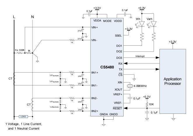
Figure 28. Typical Single-phase 2-Wire Connection
