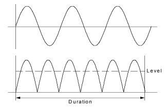
Figure 17. Sag, Swell, and Overcurrent Detect
