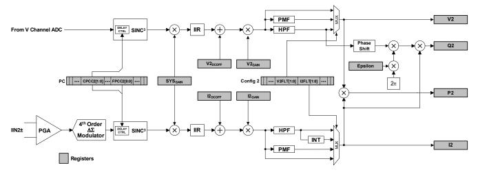
Figure 9. Signal Flow for V1, I1, P1, Q1 Measurements
