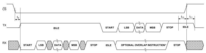
\* Reading registers during the optional overlap instruction requires the start to occur during the last byte transmitted by the part
