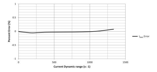
Figure 6. I<sub>RMS</sub> Load Performance
