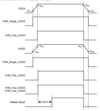
Figure 12. Power-on Reset Timing
