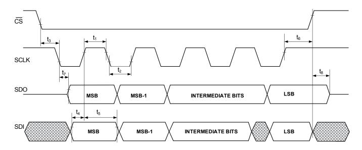
Figure 7. SPI Data and Clock Timing
