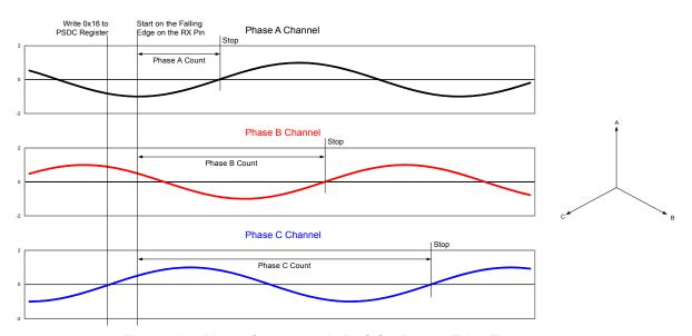
Figure 18. Phase Sequence A, B, C for Rising Edge Transition
