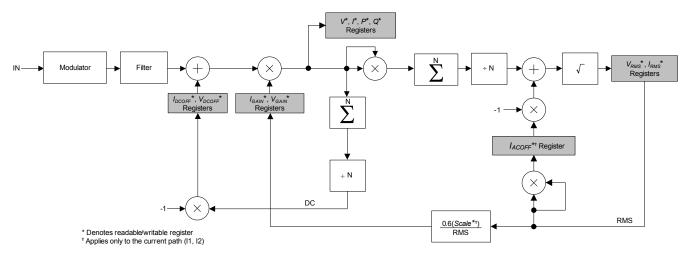
Figure 25. Calibration Data Flow
