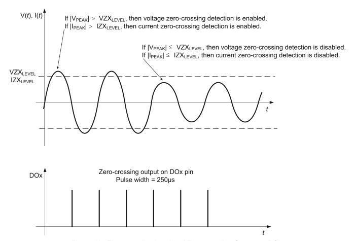
Figure 13. Zero-crossing Level and Zero-crossing Output on DOx
