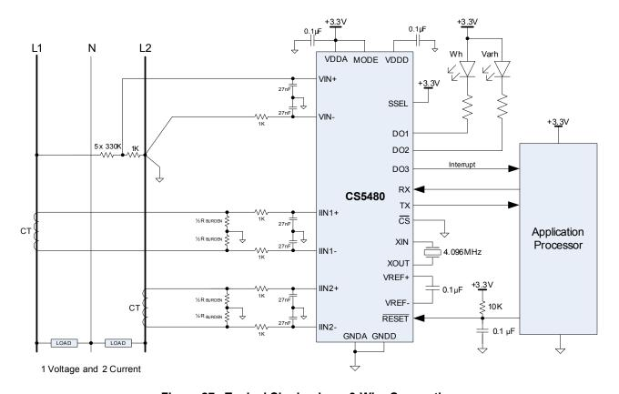
Figure 27. Typical Single-phase 3-Wire Connection
