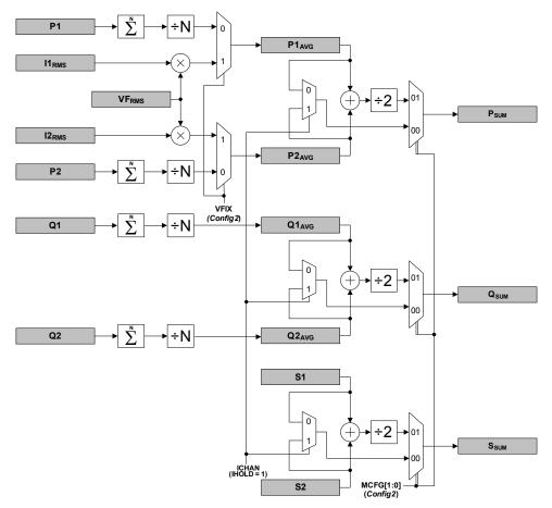
Figure 14. Channel Selection and Tamper Protection Flow
