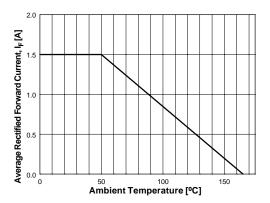
Figure 1. Forward Current Derating Curve
