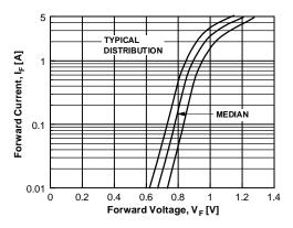
Figure 2. Forward Voltage Characteristics
