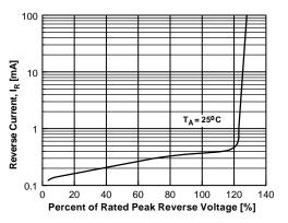
Figure 3. Reverse Current vs Reverse Voltage
