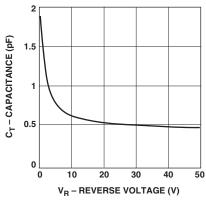
Figure 4. Total Capacitance vs. Reverse Voltage.
