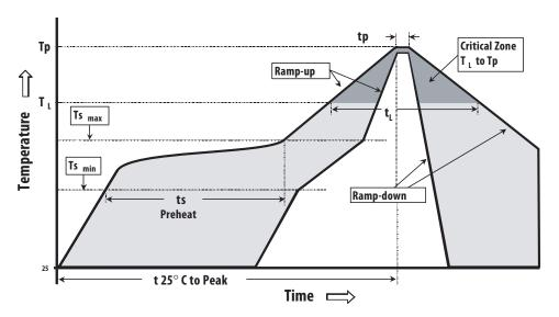
Figure 8. Surface Mount Assembly Profile.
