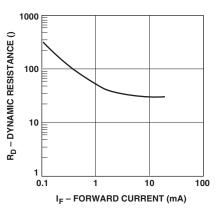
Figure 3. Dynamic Resistance vs. Forward Current.
