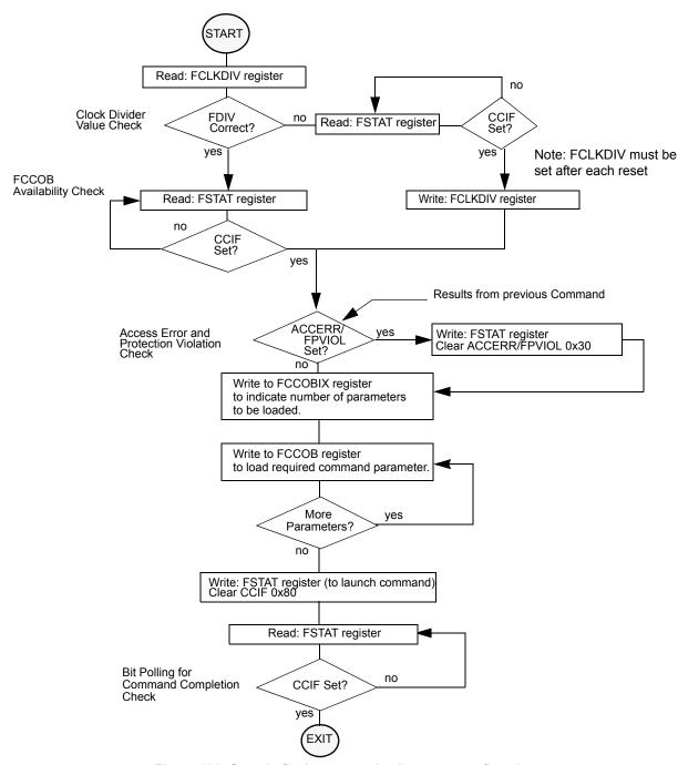
Figure 102. Generic flash command write sequence flowchart
