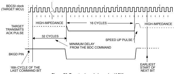
Figure 76. Target acknowledge pulse (ACK)
