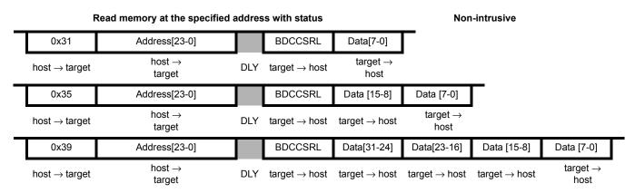
Read data at the specified memory address. The address is transmitted as three 8-bit packets (msb to lsb) immediately after the command.
