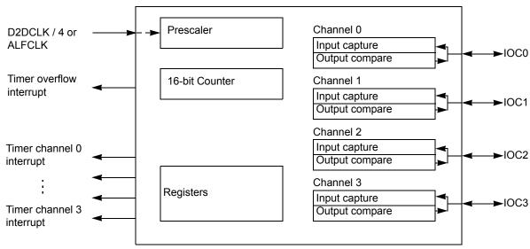
Figure 104. Timer block diagram
