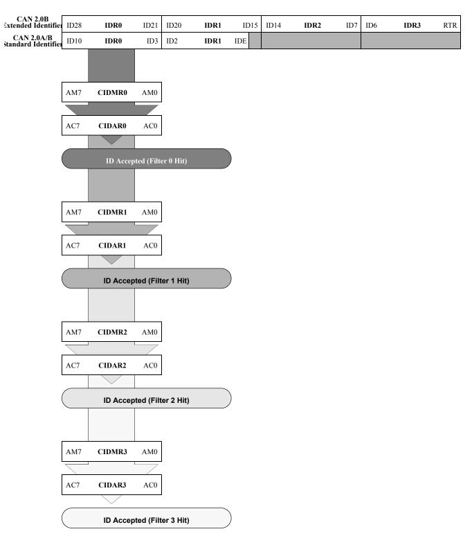
Figure 93. 8-bit maskable identifier acceptance filters
