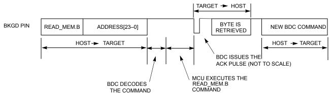
Figure 77. Handshake protocol at command level
