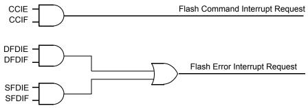
Figure 103. Flash module interrupts implementation
