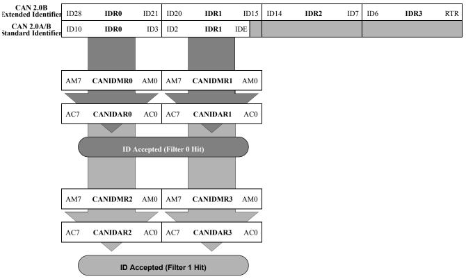
Figure 92. 16-bit maskable identifier acceptance filters
