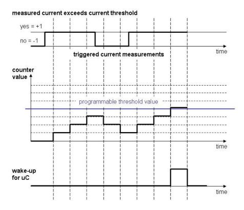
Figure 34. Current threshold - wake-up counter
