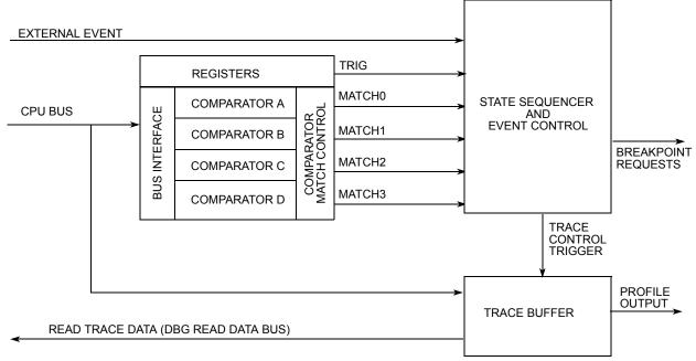
Figure 67. Debug module block diagram
