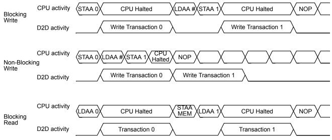
Figure 57. Blocking and non-blocking transfers.
