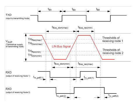
Figure 110. Definition of LIN bus timing parameters
