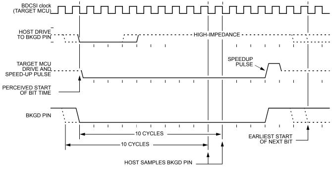
Figure 75. BDC target-to-host serial bit timing (logic 0)
