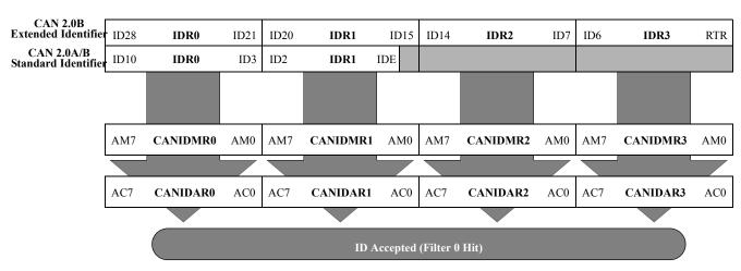
Figure 91. 32-bit maskable identifier acceptance filter
