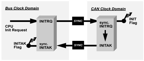
Figure 96. Initialization request/acknowledge cycle
