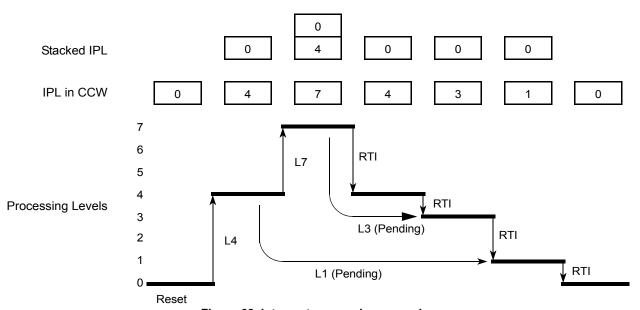
Figure 62. Interrupt processing example
