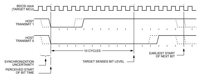
Figure 73. BDC host-to-target serial bit timing
