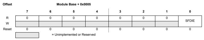
All assigned bits in the FERCNFG register are readable and writable.
