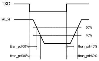
**Figure 6. LIN Transmitter Timing**
