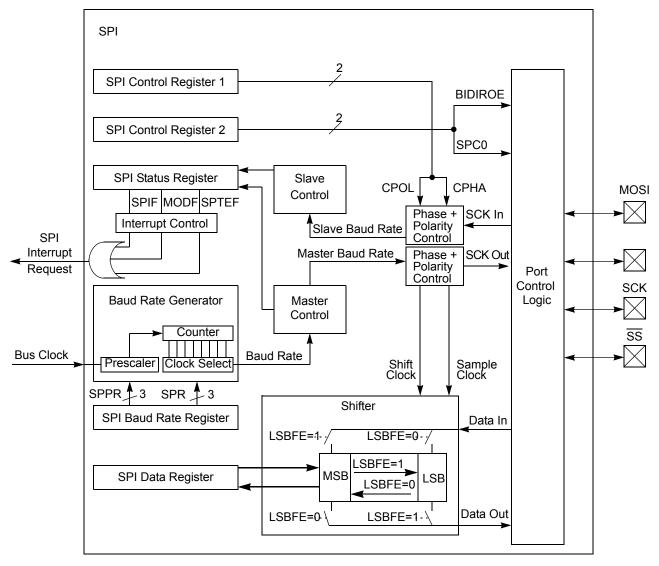
Figure 80. SPI block diagram
