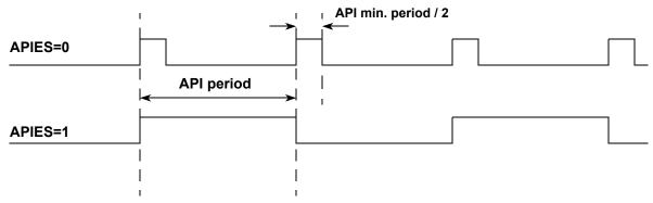
Figure 21. Waveform selected on API\_EXTCLK pin (APIEA=1, APIFE=1)
