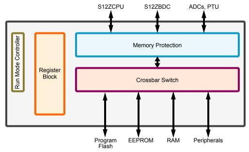
Figure 64. S12ZMMC block diagram
