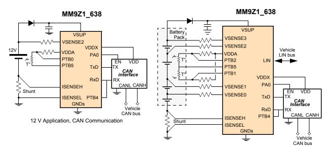
Figure 1. 12 V simplified application diagrams
