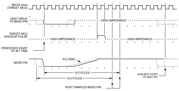
Figure 74. BDC target-to-host serial bit timing (logic 1)
