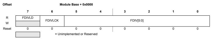
All bits in the FCLKDIV register are readable, bit 7 is not writable, bit 6 is write-once-hi and controls the writability of the FDIV field in normal mode. In Special mode, bits 6-0 are writable any number of times but bit 7 remains unwritable.
