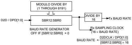
Figure 108. SCI baud rate generation
