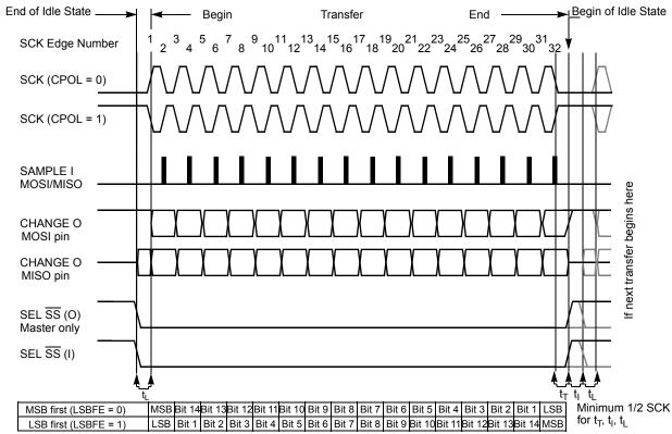
t<sub>1</sub> = Minimum leading time before the first SCK edge, not required for back-to-back transfers
