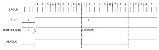
Figure 39. ALFCLK after calibration
