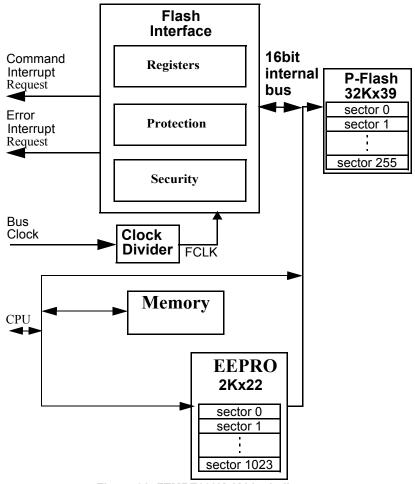
Figure 98. FTMRZ128K4K block diagram
