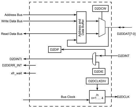
Figure 54. Die-to-die initiator (D2DI) block diagram
