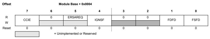
CCIE, IGNSF, FDFD, and FSFD bits are readable and writable, while remaining bits read 0 and are not writable.
