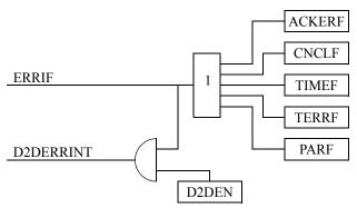
Figure 59. D2D internal interrupts
