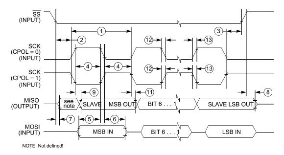
Figure 14. SPI slave timing (CPHA=1)
