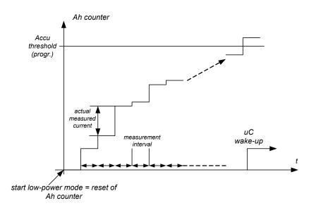
Figure 35. Ah counter function
