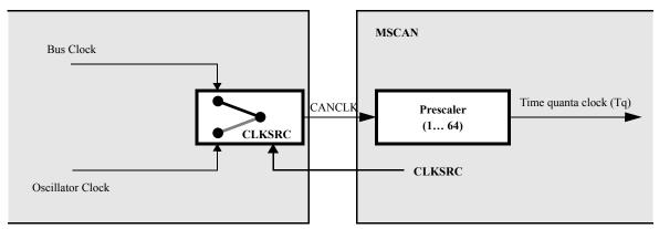
Figure 94. MSCAN clocking scheme
