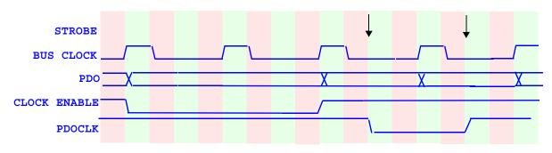
Figure 70. PDO profiling clock control
