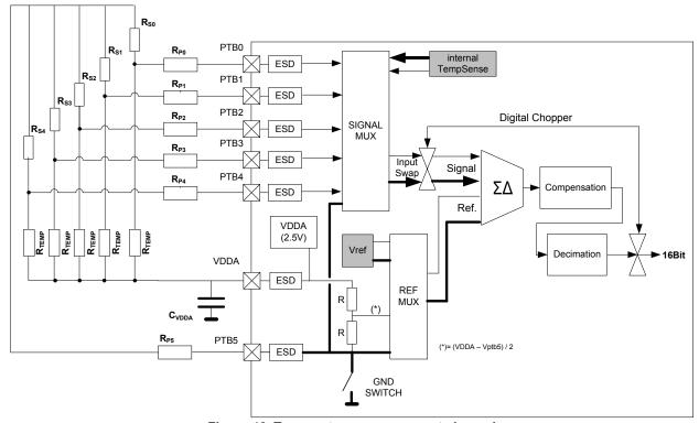
Figure 46. Temperature measurement channel
