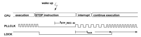
Figure 25. Stop mode using PLLCLK as bus clock
