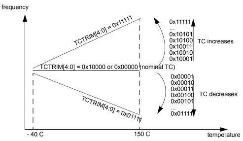
Figure 23. Influence of TCTRIM[4:0] on the temperature coefficient
