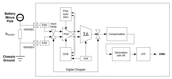
Figure 44. Current measurement channel
