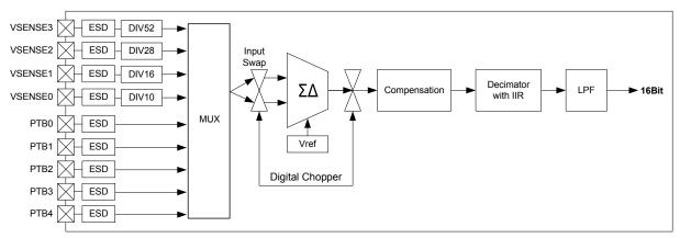
Figure 45. Voltage measurement channel
