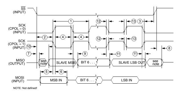
Figure 13. SPI slave timing (CPHA=0)
