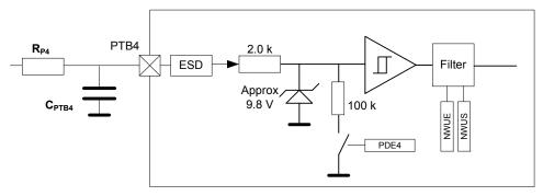
Figure 51. PTB4 input structure (typical values indicated)
