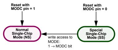
Figure 65. Mode transition diagram
