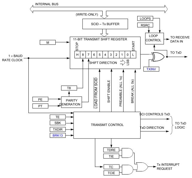
Figure 106. SCI transmitter block diagram
