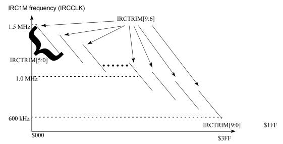
Figure 22. IRC1M frequency trimming diagram
