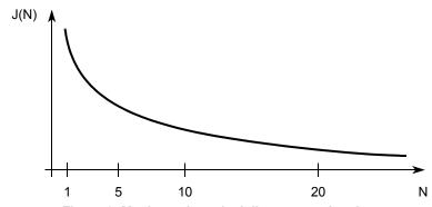
Figure 9. Maximum bus clock jitter approximation
