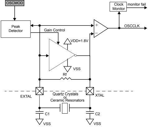
Figure 20. XOSCLCP block diagram
