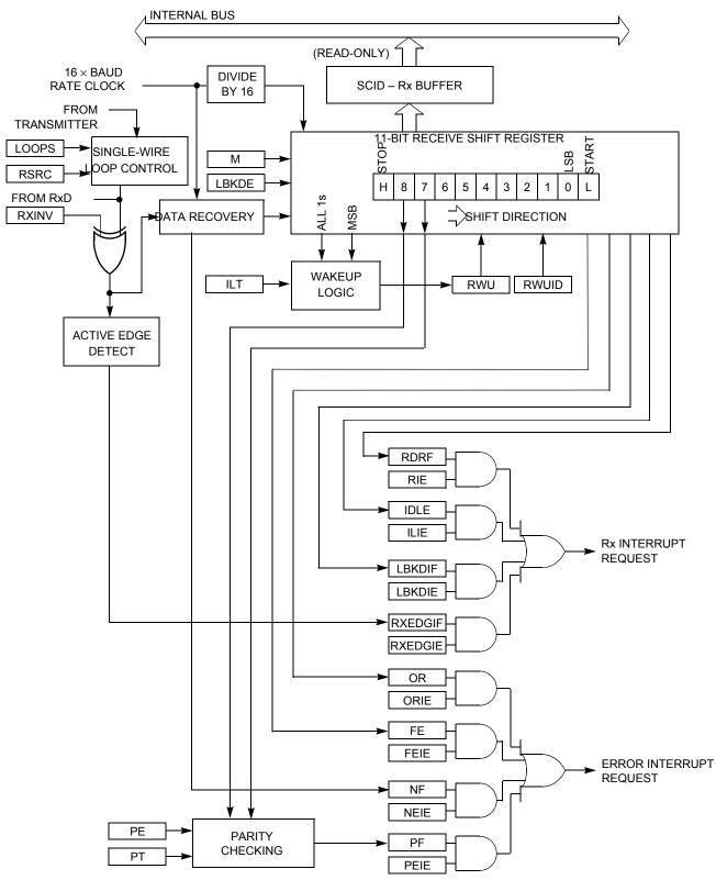
Figure 107. SCI receiver block diagram
