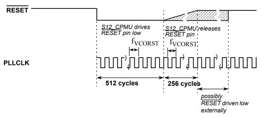
Figure 28. RESET timing
