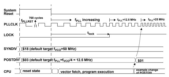
Figure 24. Startup of clock system after reset
