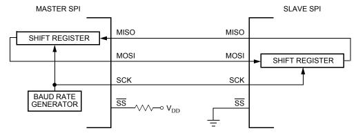
Figure 83. Master/slave transfer block diagram
