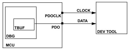
Figure 69. Profiling output interface
