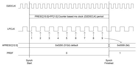
Figure 38. ALF clock calibration procedure during normal mode
