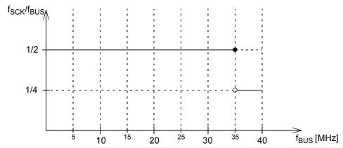
Figure 12. Derating of maximum  $f_{\mbox{\footnotesize SCK}}$  to  $f_{\mbox{\footnotesize BUS}}$  ratio in master mode
