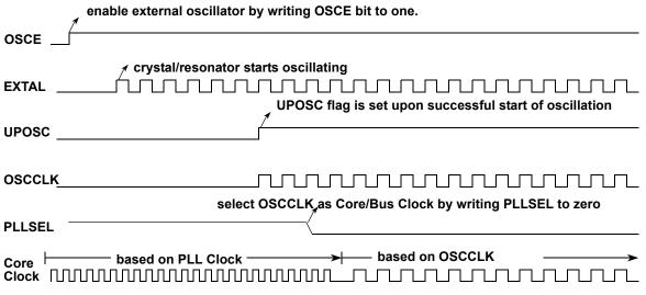
Figure 27. Enabling the external oscillator
