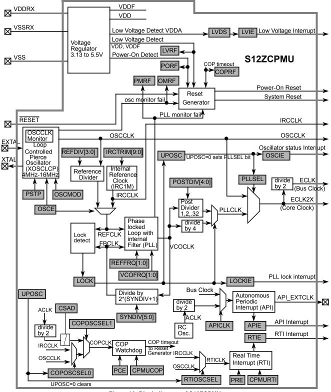
Figure 19. Block diagram of S12ZCPMU
