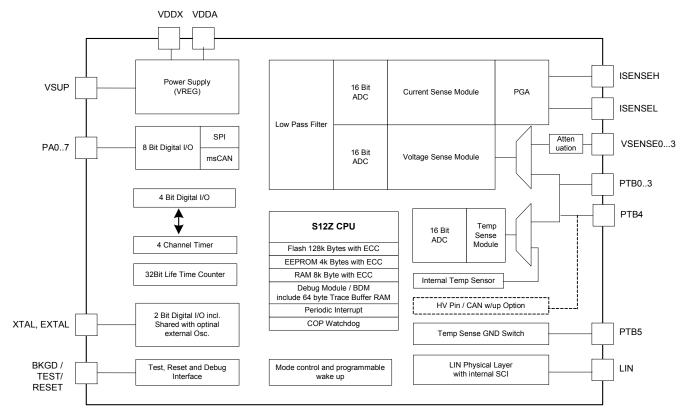
Figure 15. Simplified block diagram
