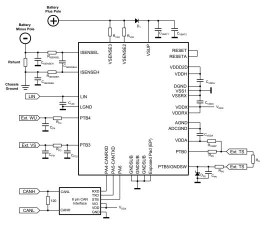
Note: Module GND connected to Battery Minus or Chassis Ground – based on configuration
