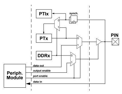
Figure 53. Illustration of I/O pin functionality
