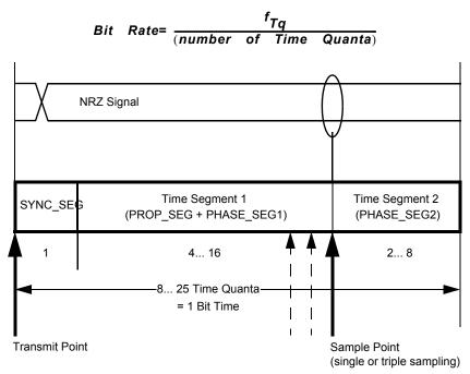
Figure 95. Segments within the bit time
