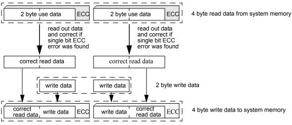
Figure 63. 2 Byte non-aligned write access
