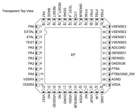
Figure 4. MM9Z1\_638 pin connections
