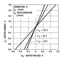
Figure 8 Typical Output Leakage Current vs. Temperature
