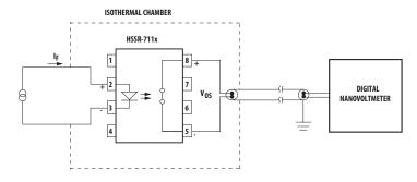
Figure 20 Burn-In Circuit
