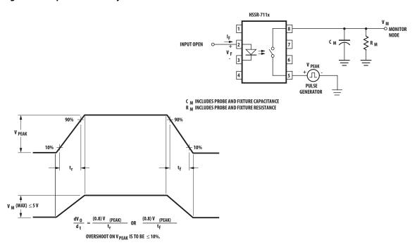
**Figure 18 Input-Output Transient Rejection Test Circuit**
