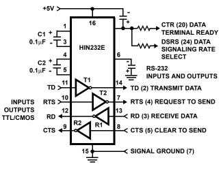
FIGURE 7. SIMPLE DUPLEX RS-232 PORT WITH CTS/RTS HANDSHAKING
