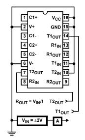
FIGURE 2. POWER-OFF SOURCE RESISTANCE CONFIGURATION
