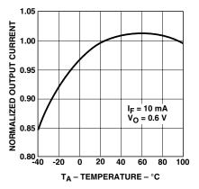
Figure 2. Normalized output current vs. temperature.
