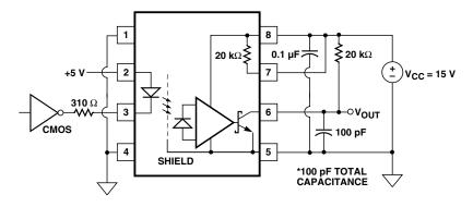
Figure 15. Recommended LED drive circuit.
