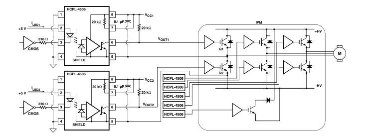
Figure 24. Typical application circuit.
