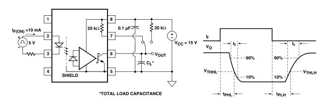
Figure 6. Propagation delay test circuit.
