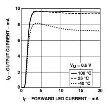
Figure 1. Typical transfer characteristics.
