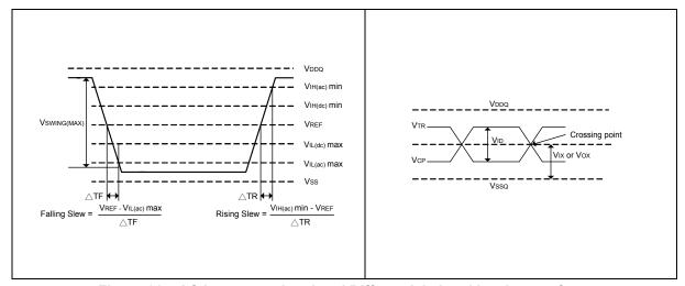
Figure 28—AC input test signal and Differential signal levels waveform
