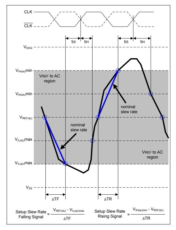
Figure 20 —Illustration of nominal slew rate for tis
