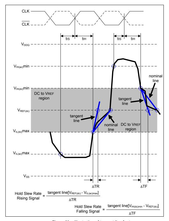
Figure 23 —Illustration of tangent line for till
