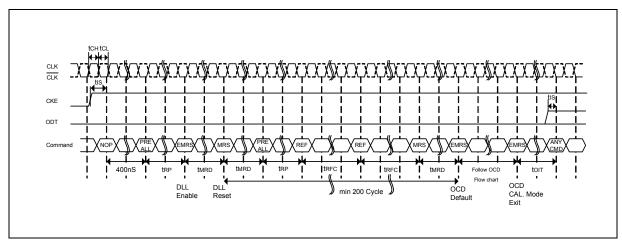
Figure 1—Initialization sequence after power-up
