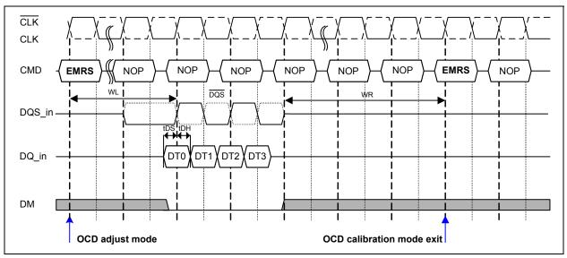
Figure 7—OCD Adjust Mode
