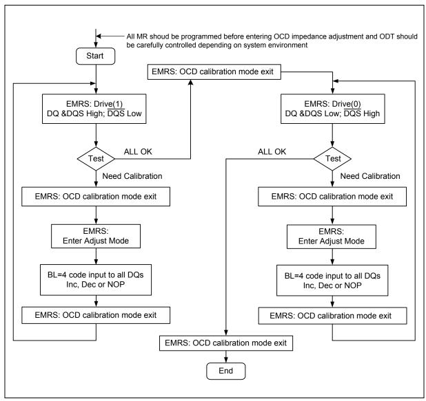
Figure 6—OCD Impedance Adjustment Flow Chart
