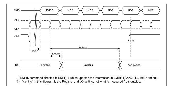
Figure 10—ODT update delay timing - tMOD
