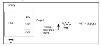
Figure 16 — AC timing reference load
