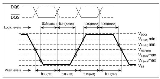
Figure 19 — Differential input waveform timing - tDS and tDH
