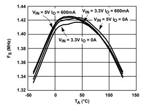
FIGURE 5. F<sub>S</sub> vs JUNCTION TEMPERATURE (PWM MODE)
