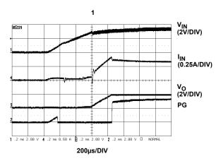
FIGURE 10. START-UP AT  $I_0 = 600 \text{mA}$
