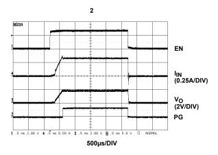
FIGURE 11. ENABLE AND SHUTDOWN
