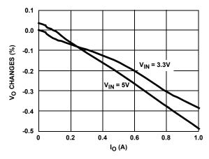
FIGURE 6. LOAD REGULATIONS (PWM MODE)
