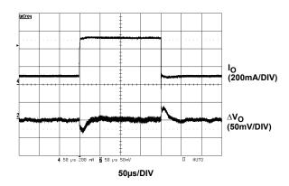
FIGURE 18. PWM LOAD TRANSIENT RESPONSE (100mA TO 500mA)
