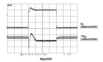
FIGURE 16. LOAD TRANSIENT RESPONSE (22mA TO 600mA)
