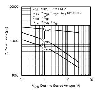
Fig 10. Typical Capacitance vs. Drain-to-Source Voltage
