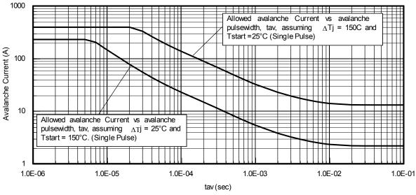
Fig 16. Typical Avalanche Current vs. Pulse Width
