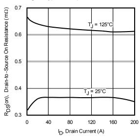
Fig. 4 Typical On-Resistance vs. Drain Current
