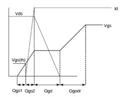
Fig 19b. Gate Charge Waveform
