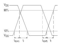
Fig 20b. Switching Time Waveforms
