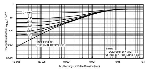
Fig 15. Maximum Effective Transient Thermal Impedance, Junction-to-Case
