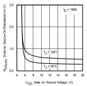
Fig. 3 Typical On-Resistance vs. Gate Voltage
