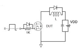
Fig 19a. Gate Charge Test Circuit
