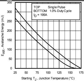
Fig 17. Maximum Avalanche Energy vs. Temperature
