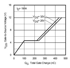
Fig 11. Typical Gate Charge vs.
