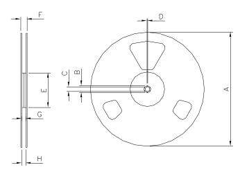
NOTE: Controlling dimensions in mm Std reel quantity is 4000 parts, ordered as AUIRF8739L2TR.
