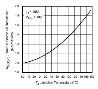
Fig 6. Normalized On-Resistance vs. Temperature
