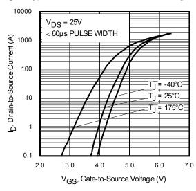
Fig 5. Transfer Characteristics
