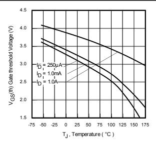
**Fig. 7** Typical Threshold Voltage vs. Junction Temperature
