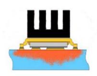
Mounted to a PCB with small clip heatsink (still air)
