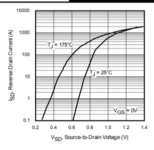
Fig 8. Typical Source-Drain Diode Forward Voltage
