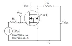
Fig 20a. Switching Time Test Circuit
