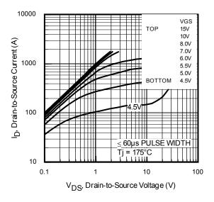
Fig. 2 Typical Output Characteristics
