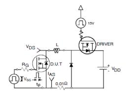
Fig 18a. Unclamped Inductive Test Circuit
