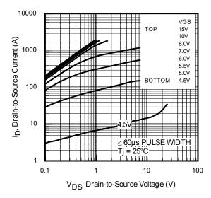
Fig. 1 Typical Output Characteristics
