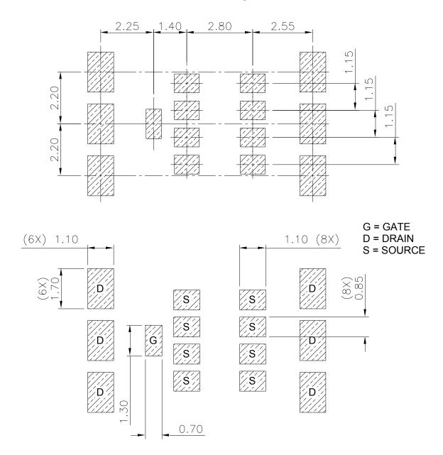
Note: For the most current drawing please refer to IR website at <a href="http://www.irf.com/package/">http://www.irf.com/package/</a>
