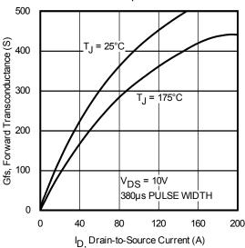
Fig 9. Typical Forward Transconductance vs. Drain Current
