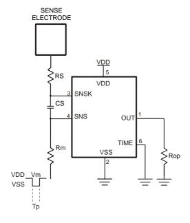
To ensure the pulse is detected it must be present for a time greater than the burst length as shown in Table 3.6.
