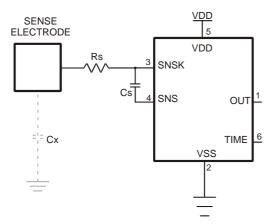
For optimum noise immunity, the electrode should only be connected to the SNSK pin.
