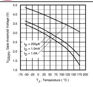
Fig 16. Threshold Voltage vs. Temperature
