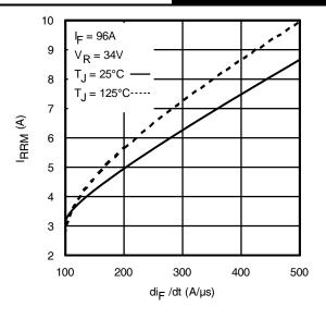
Fig. 17 - Typical Recovery Current vs. dif/dt
