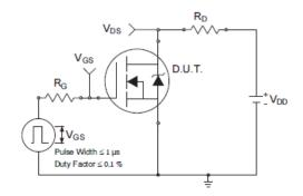
Fig 23a. Switching Time Test Circuit
