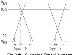
Fig 23b. Switching Time Waveforms
