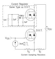
Fig 24a. Gate Charge Test Circuit
