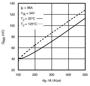
Fig. 19 - Typical Stored Charge vs. dif/dt
