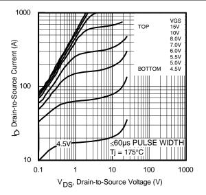
Fig. 2 Typical Output Characteristics
