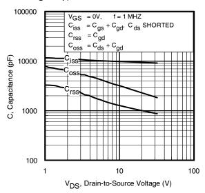
Fig 5. Typical Capacitance vs. Drain-to-Source Voltage
