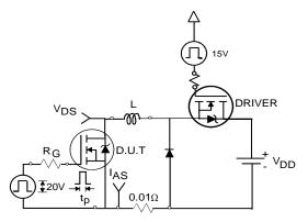
Fig 22a. Unclamped Inductive Test Circuit
