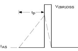
Fig 22b. Unclamped Inductive Waveforms
