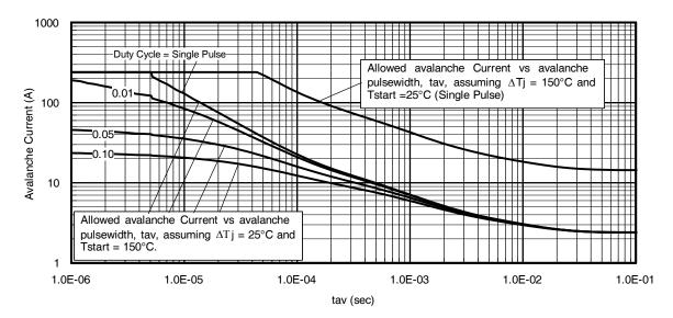
Fig 14. Avalanche Current vs. Pulse width
