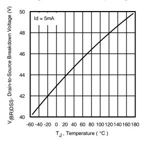
Fig 10. Drain-to-Source Breakdown Voltage
