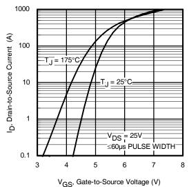
Fig. 3 Typical Transfer Characteristics
