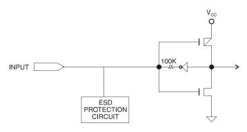
Figure 8-2. I/O Diagram
