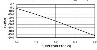
ATMEL ATF22V10C/CQ OUTPUT SINK CURRENT VS. SUPPLY VOLTAGE ( $V_{OL} = 0.5V$ )
