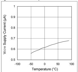
Figure 5. Supply Current VCCA vs. Temperature
