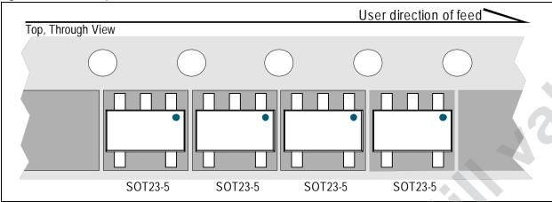
Figure 20. AS1922 Tape&Reel Pin1 Orientation
