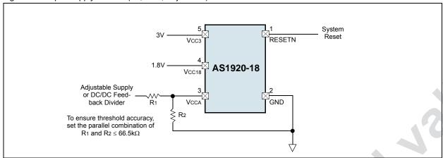
Figure 14. Dual-Supply Monitor (3V and 1.8V; Disable Vcca Input)
