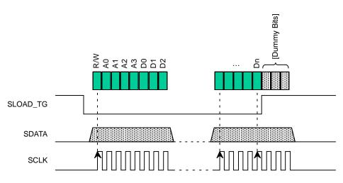
Figure 3. KSC-1000 Initialization Timing
