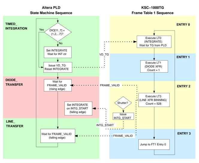
Figure 10. Dual Channel Mode Timing Sequence
