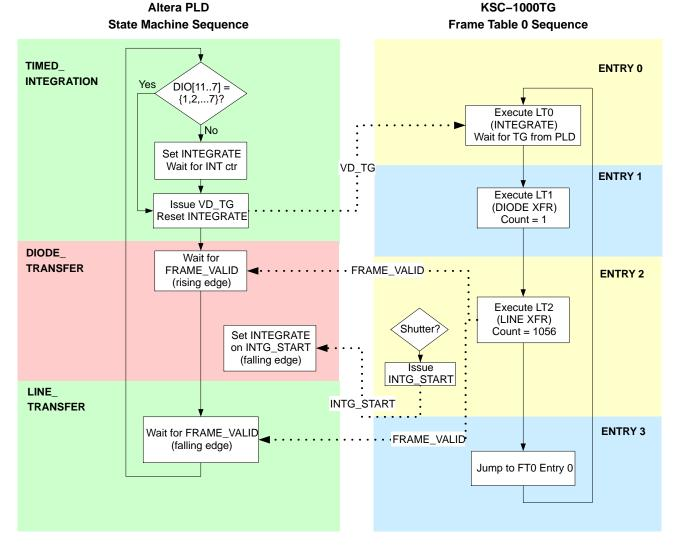
Figure 8. Single and Dual Channel Mode Timing Sequence
