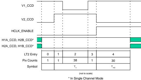
Polarity is reversed for H2B\_CCD and H1B\_CCD for Dual Channel Mode
