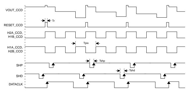
Figure 14. Binning Mode Horizontal Timing
