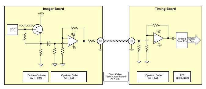
Figure 19. Video Signal Path Block Diagram
