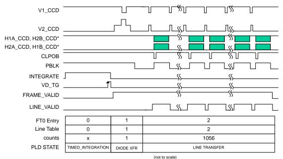
\* In Single Channel Mode Polarity is reversed for H2B\_CCD and H1B\_CCD for Dual Channel Mode
