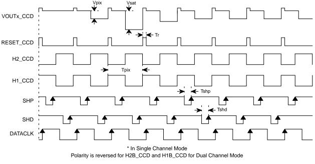
Figure 13. Horizontal Timing
