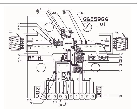
Figure 4. Layout of Test Evaluation Board (RMBA09501-TD, G657471)
