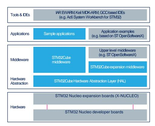
Compatibility with multiple Development Environments - The STM32 Open Development Environment is compatible with a number of IDEs including IAR EWARM, Keil MDK, and GCC-based environments. Users can choose from three IDEs from leading vendors, which are free of charge and deployed in close cooperation with ST. These include Eclipse-based IDEs such as Ac6 System Workbench for STM32 and the MDK-ARM environment.
