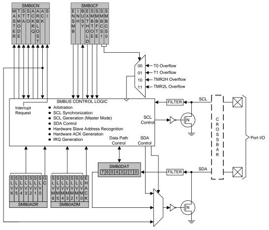
Figure 30.1. SMBus Block Diagram
