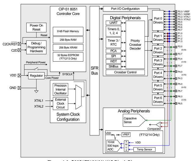
Figure 1.6. C8051F712/13/14/15 Block Diagram
