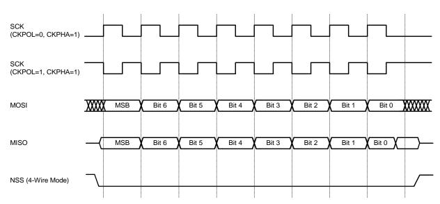
Figure 31.7. Slave Mode Data/Clock Timing (CKPHA = 1)
