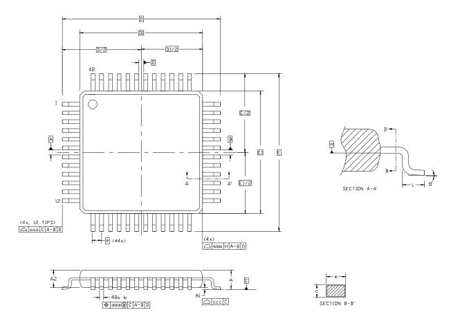
Figure 5.1. TQFP-48 Package Drawing
