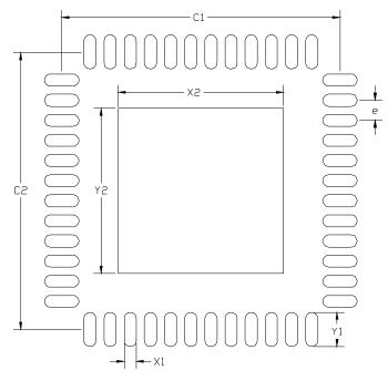
Figure 6.2. QFN-48 PCB Land Pattern
