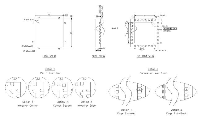
Figure 7.1. QFN-32 Package Drawing
