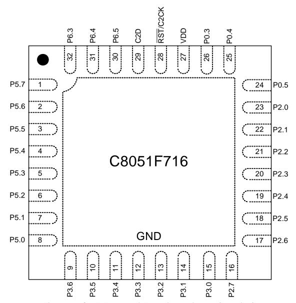
Figure 3.4. C8051F716-GM QFN32 Pinout Diagram (Top View)
