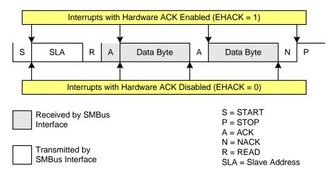
Figure 30.6. Typical Master Read Sequence
