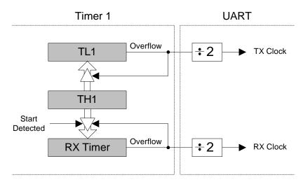
Figure 32.2. UARTO Baud Rate Logic
