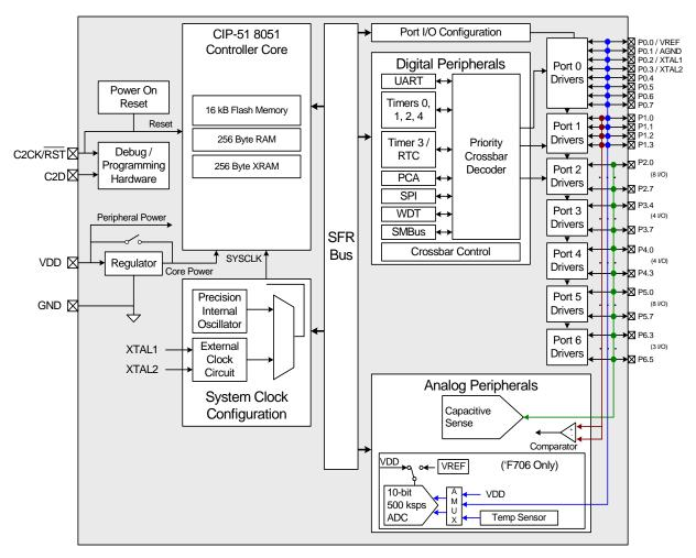
Figure 1.4. C8051F706/07 Block Diagram
