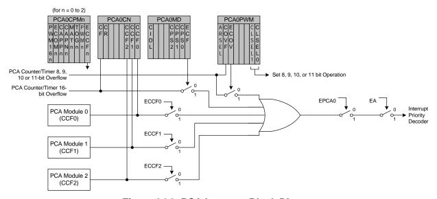
Figure 34.3. PCA Interrupt Block Diagram
