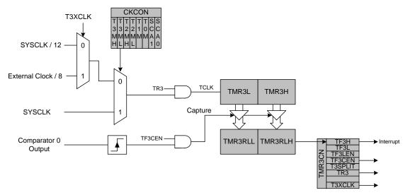
Figure 33.9. Timer 3 Capture Mode Block Diagram
