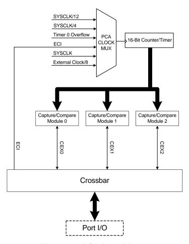
Figure 34.1. PCA Block Diagram
