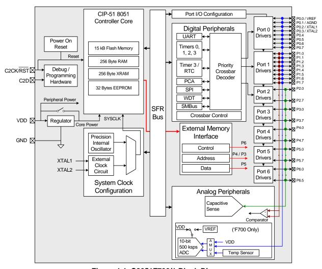
Figure 1.1. C8051F700/1 Block Diagram
