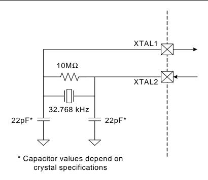
Figure 27.2. External 32.768 kHz Quartz Crystal Oscillator Connection Diagram
