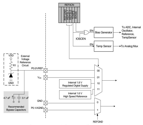
Figure 12.1. Voltage Reference Functional Block Diagram
