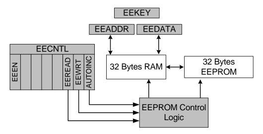
Figure 23.1. EEPROM Block Diagram
