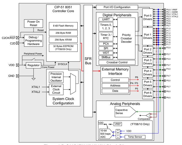
Figure 1.5. C8051F708/09/10/11 Block Diagram
