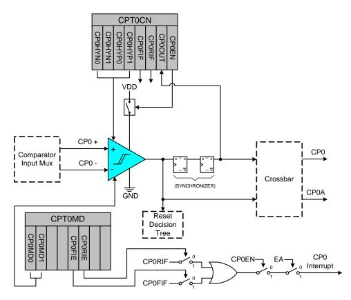
Figure 14.1. Comparator Functional Block Diagram
