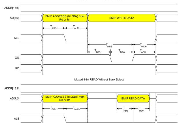
Figure 18.8. Multiplexed 8-Bit MOVX without Bank Select Timing
