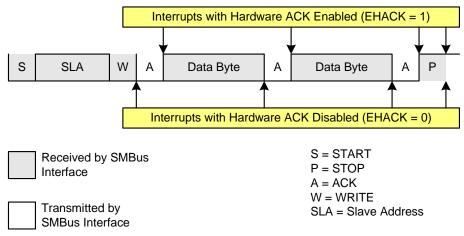
Figure 30.7. Typical Slave Write Sequence
