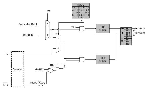
Figure 33.3. T0 Mode 3 Block Diagram
