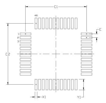
Figure 5.2. TQFP-48 PCB Land Pattern
