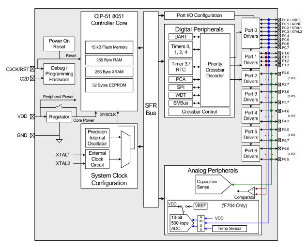
Figure 1.3. C8051F704/5 Block Diagram
