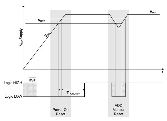
Figure 25.2. Power-On and V<sub>DD</sub> Monitor Reset Timing
