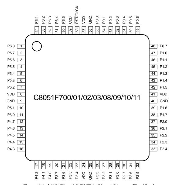
Figure 3.1. C8051F7xx-GQ TQFP64 Pinout Diagram (Top View)
