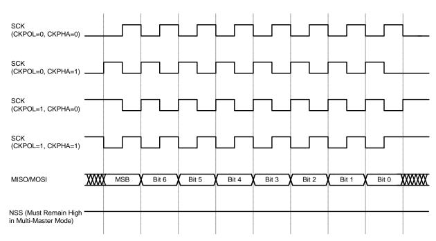
Figure 31.5. Master Mode Data/Clock Timing
