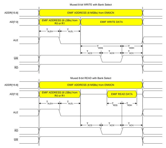
Figure 18.9. Multiplexed 8-Bit MOVX with Bank Select Timing
