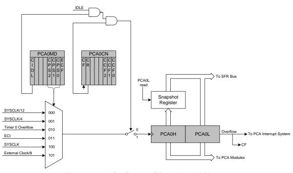
Figure 34.2. PCA Counter/Timer Block Diagram
