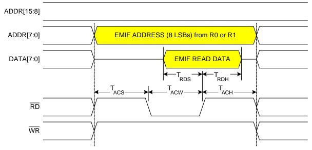
Figure 18.5. Non-multiplexed 8-bit MOVX without Bank Select Timing
