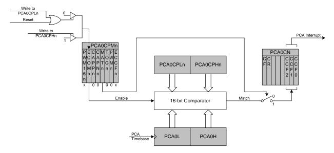
Figure 34.5. PCA Software Timer Mode Diagram
