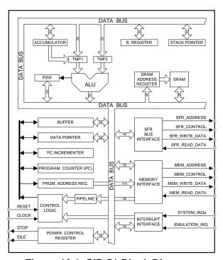
Figure 16.1. CIP-51 Block Diagram
