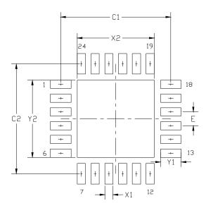
Figure 8.2. QFN-24 Recommended PCB Land Pattern
