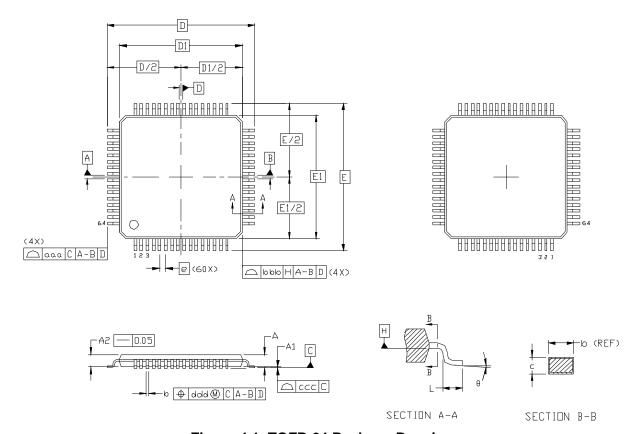
Figure 4.1. TQFP-64 Package Drawing
