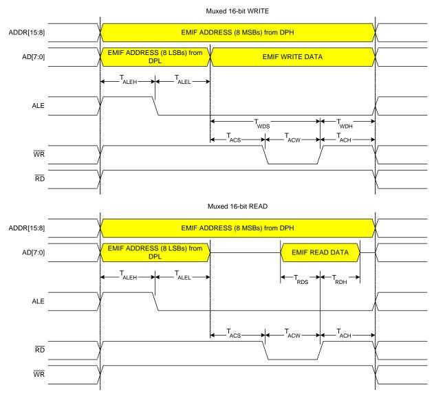
Figure 18.7. Multiplexed 16-bit MOVX Timing
