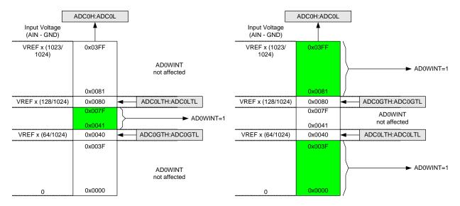
Figure 10.4. ADC Window Compare Example: Right-Justified Data
