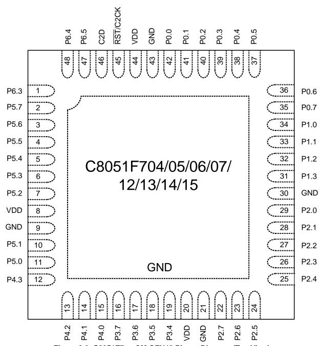
Figure 3.3. C8051F7xx-GM QFN48 Pinout Diagram (Top View)
