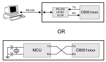
Figure 32.3. UART Interconnect Diagram
