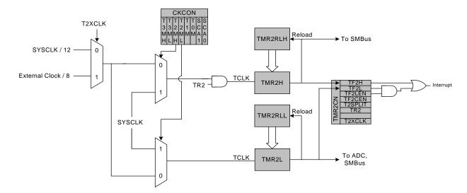
Figure 33.5. Timer 2 8-Bit Mode Block Diagram
