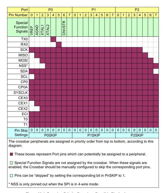
Figure 28.4. Crossbar Priority Decoder—Possible Pin Assignments
