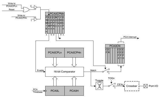
Figure 34.6. PCA High-Speed Output Mode Diagram
