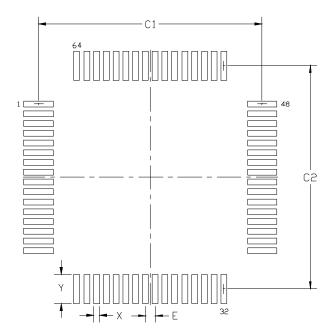
Figure 4.2. TQFP-64 PCB Land Pattern
