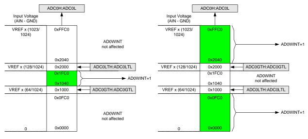
Figure 10.5. ADC Window Compare Example: Left-Justified Data
