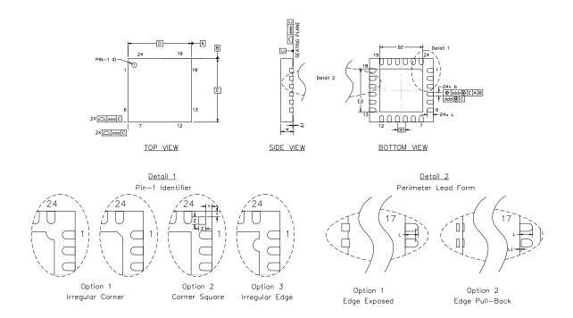
Figure 8.1. QFN-24 Package Drawing
