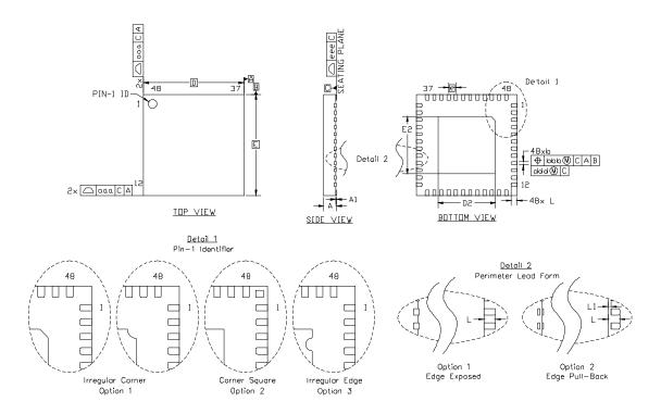
Figure 6.1. QFN-48 Package Drawing
