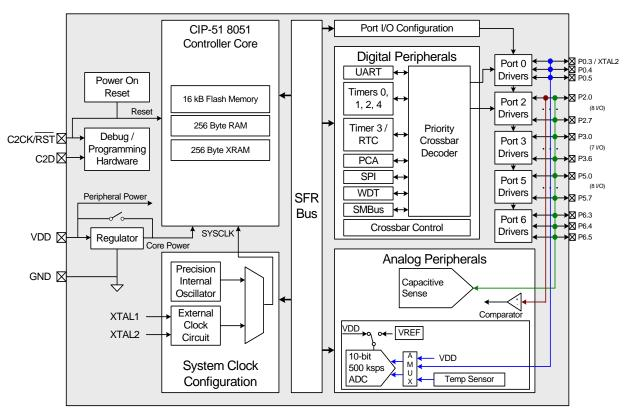
Figure 1.7. C8051F716 Block Diagram
