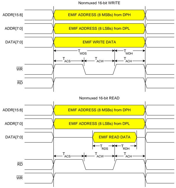
Figure 18.4. Non-multiplexed 16-bit MOVX Timing
