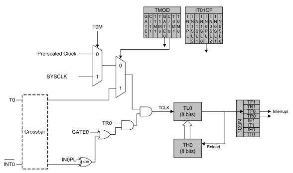
Figure 33.2. T0 Mode 2 Block Diagram
