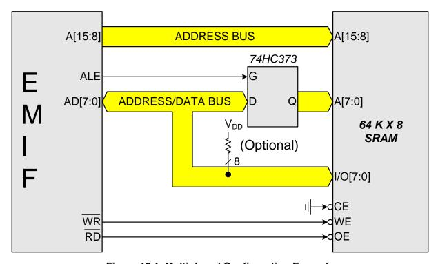
Figure 18.1. Multiplexed Configuration Example
