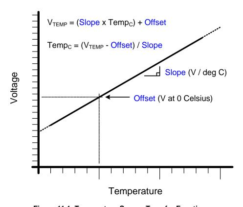
Figure 11.1. Temperature Sensor Transfer Function
