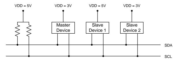
Figure 30.2. Typical SMBus Configuration
