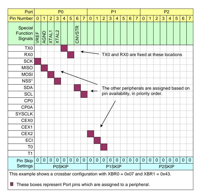
Figure 28.5. Crossbar Priority Decoder in Example Configuration—No Pins Skipped
