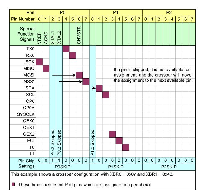
Figure 28.6. Crossbar Priority Decoder in Example Configuration—3 Pins Skipped
