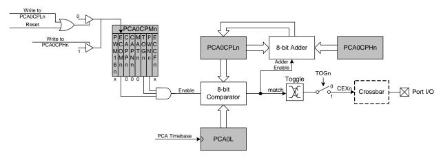
Figure 34.7. PCA Frequency Output Mode
