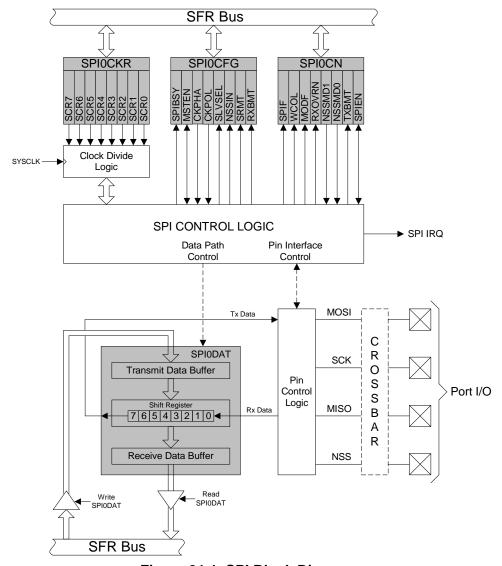
Figure 31.1. SPI Block Diagram
