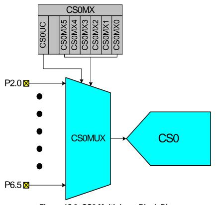
Figure 15.3. CS0 Multiplexer Block Diagram
