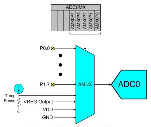
Figure 10.6. ADC0 Multiplexer Block Diagram
