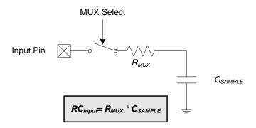
Note: See electrical specification tables for  $R_{\text{MUX}}$  and  $C_{\text{SAMPLE}}$  parameters.
