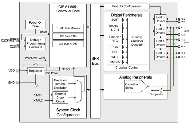
Figure 1.8. C8051F717 Block Diagram
