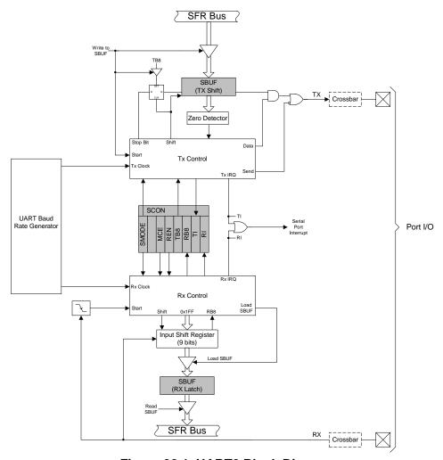
Figure 32.1. UARTO Block Diagram
