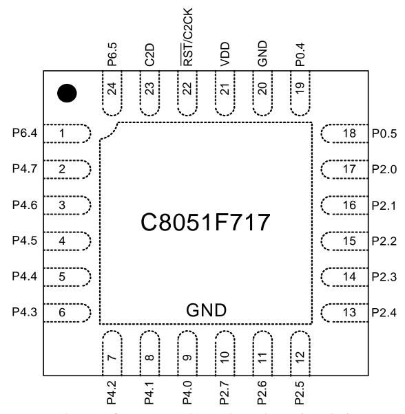
Figure 3.5. C8051F717-GM QFN24 Pinout Diagram (Top View)
