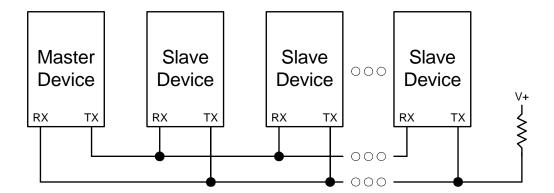
Figure 32.6. UART Multi-Processor Mode Interconnect Diagram
