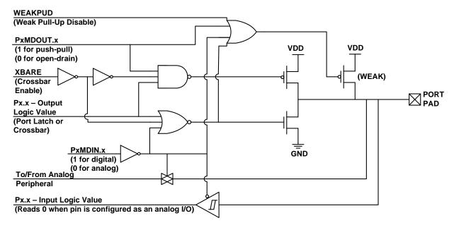
Figure 28.2. Port I/O Cell Block Diagram
