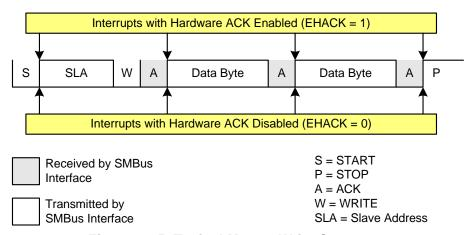
Figure 30.5. Typical Master Write Sequence
