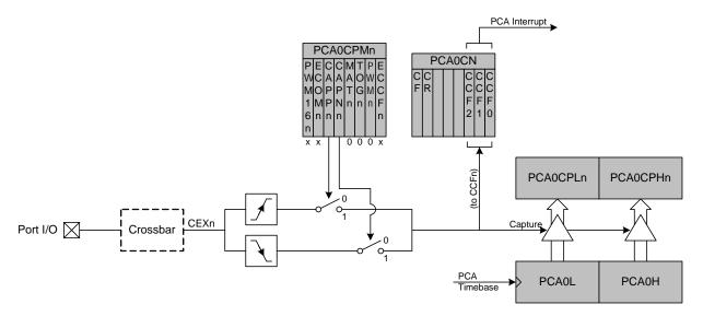
Figure 34.4. PCA Capture Mode Diagram
