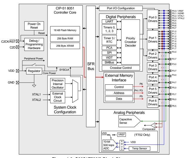
Figure 1.2. C8051F702/3 Block Diagram
