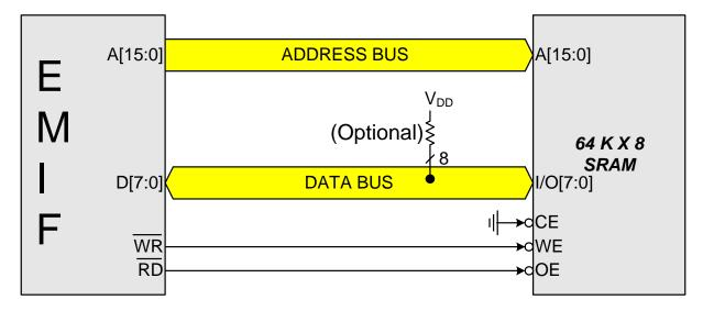
Figure 18.2. Non-multiplexed Configuration Example
