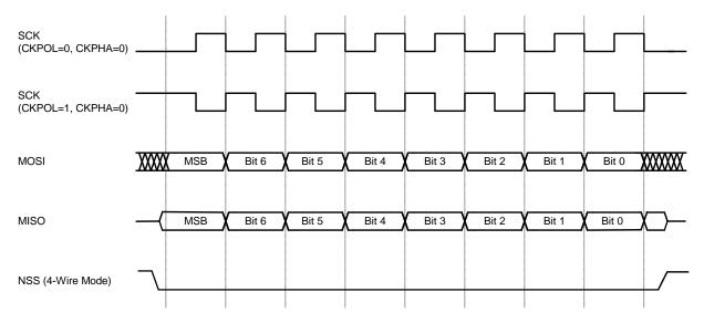
Figure 31.6. Slave Mode Data/Clock Timing (CKPHA = 0)
