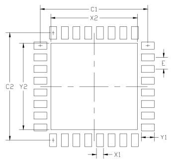
Figure 7.2. QFN-32 Recommended PCB Land Pattern
