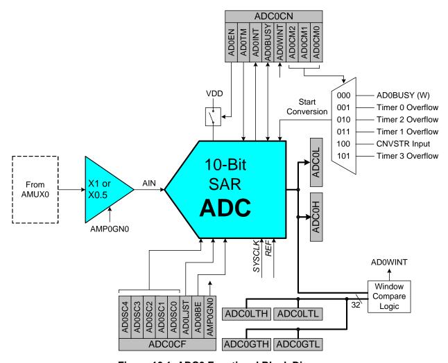
Figure 10.1. ADC0 Functional Block Diagram
