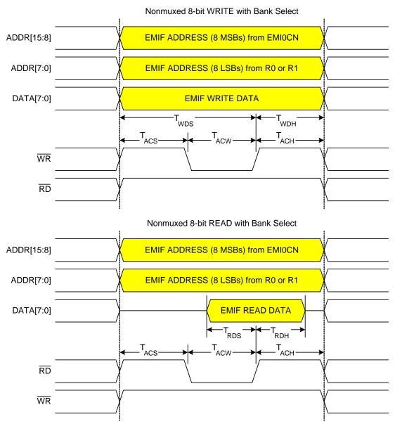
Figure 18.6. Non-Multiplexed 8-Bit MOVX with Bank Select Timing
