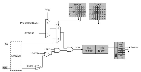
Figure 33.1. T0 Mode 0 Block Diagram
