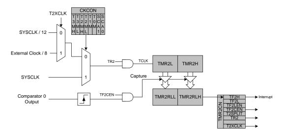
Figure 33.6. Timer 2 Capture Mode Block Diagram
