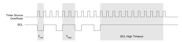
Figure 30.4. Typical SMBus SCL Generation
