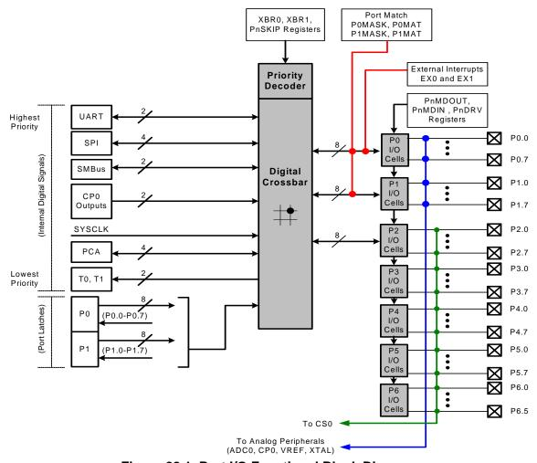
Figure 28.1. Port I/O Functional Block Diagram
