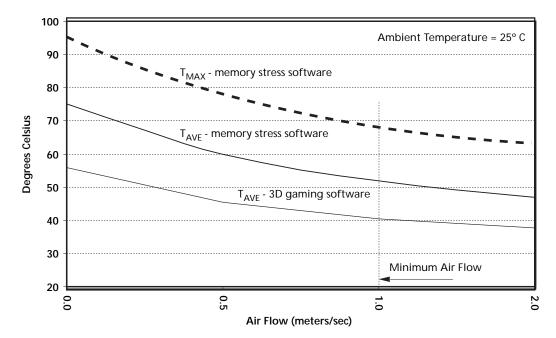
Notes: 1. Micron Technology, Inc. recommends a minimum air flow of 1 meter/second (~197 LFM) across all modules when installed in a system.
