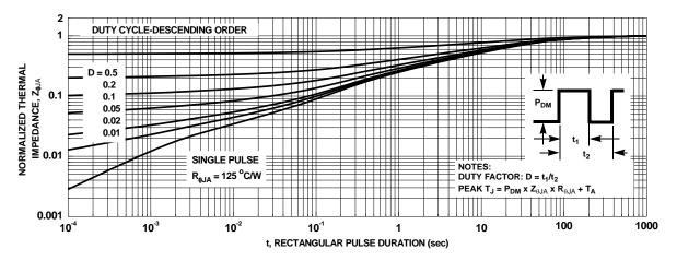
Figure 13. Junction-to-Ambient Transient Thermal Response Curve
