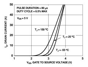
Figure 5. Transfer Characteristics
