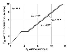
Figure 7. Gate Charge Characteristics
