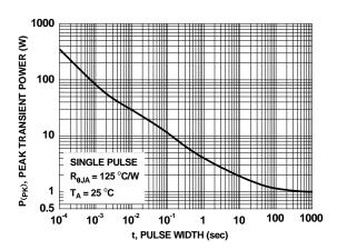
Figure 12. Single Pulse Maximum Power Dissipation
