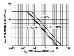
Figure 9. Unclamped Inductive Switching Capability
