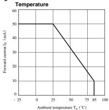
Fig. 1 Forward Current vs. Ambient
