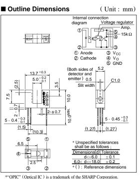
\*"OPIC" (Optical IC) is a trademark of the SHARP Corporation. An OPIC consists of a light-detecting element and signalprocessing circuit integrated onto a single chip.
